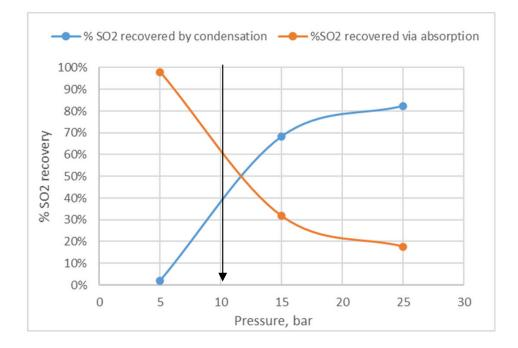
Although increasing pressure at around 10 barg in order not to be too detrimental for the SO3 decomposition, the amount of water is too high for the downstream section.
