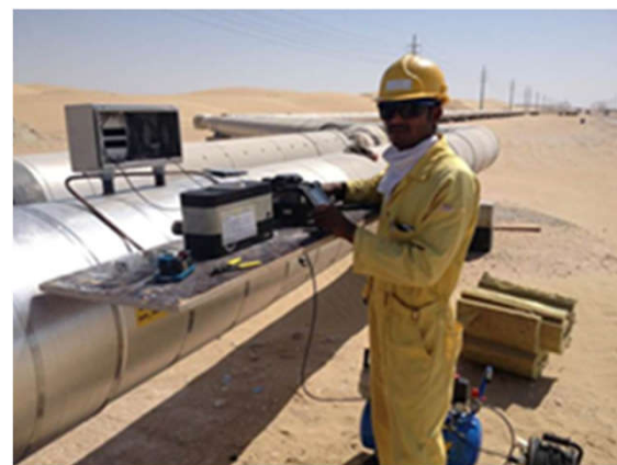
Molten sulphur in heated pipelines (~140 °C)
