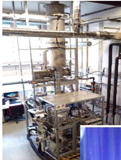
Sulphur combustor for gas turbines
